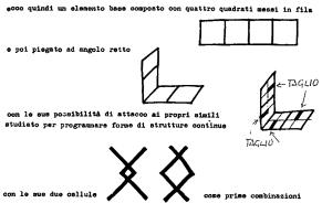
Explanatory drawings on the principle of continuous structures from "Codice Ovvio", Bruno Munari®1972
